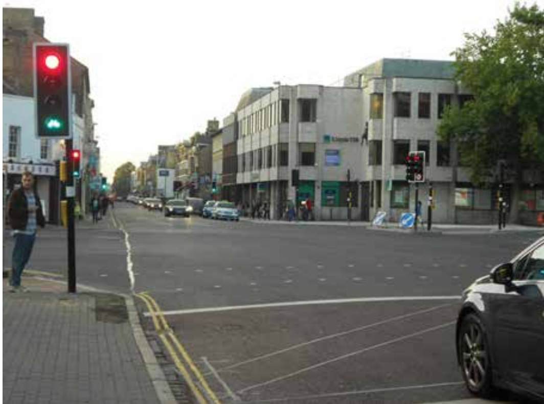
Photo 6.26 - Early Start Cycle Filter at ASL, Cambridge
