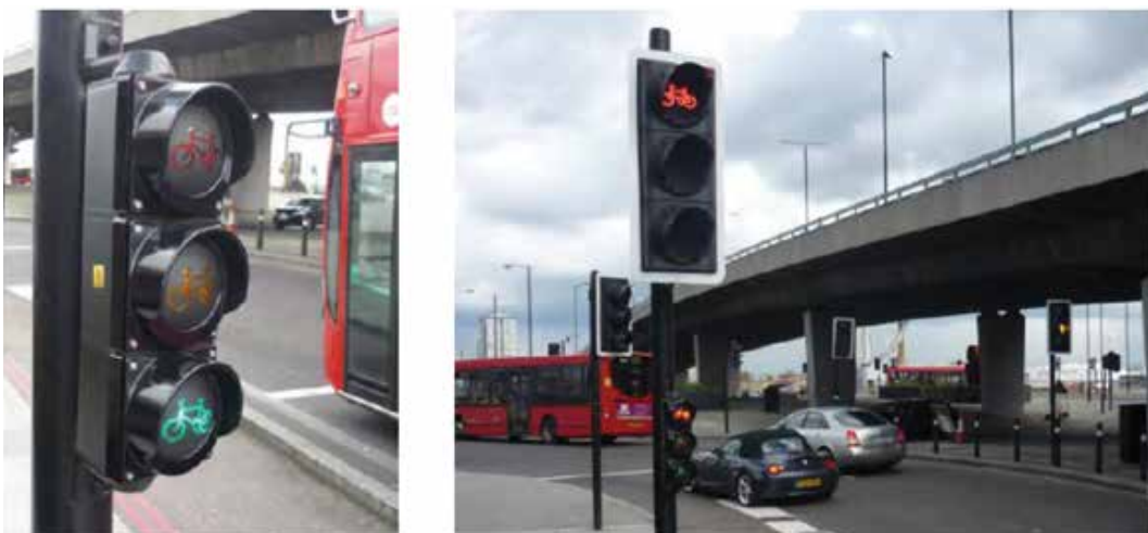
Photo 6.28 – Low Level Cycle Signals and Red Cycle Aspect on trial at Bow Roundabout, London.*
