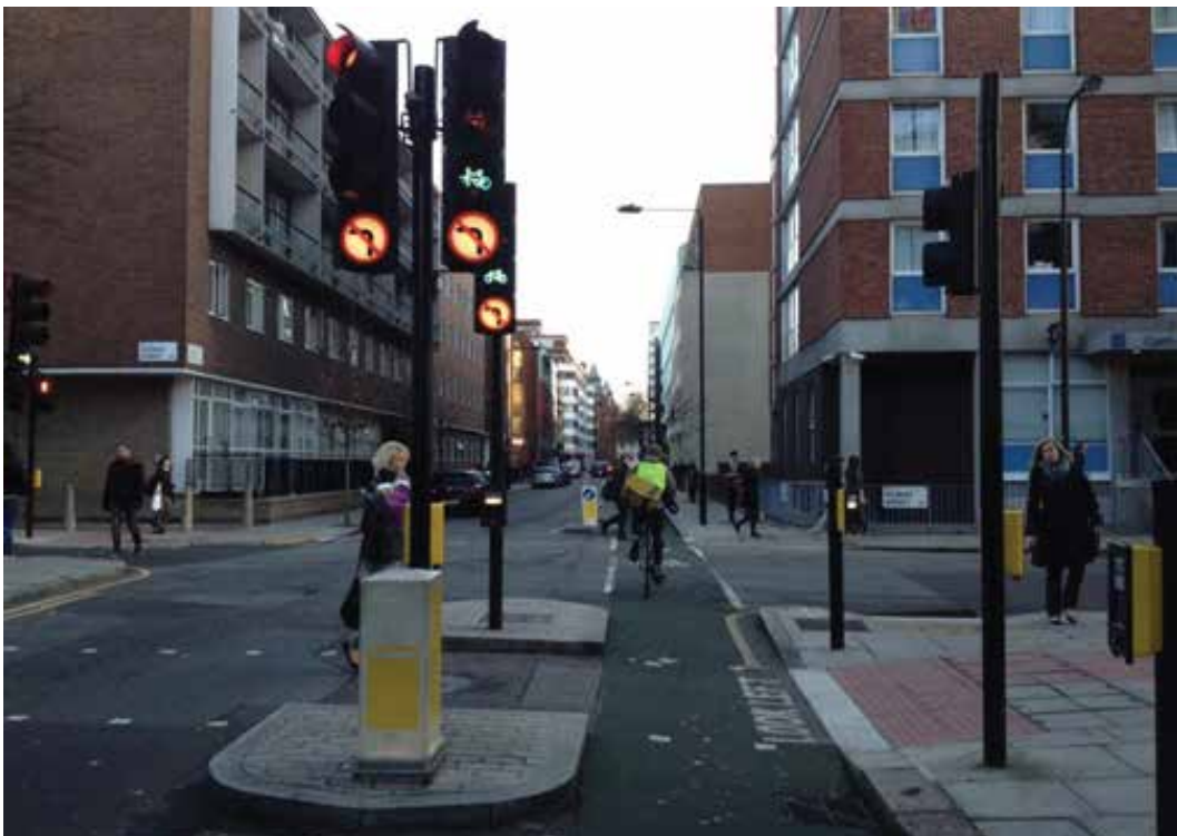
Photo 6.28 – Low Level Cycle Signals and Red Cycle Aspect on trial at Bow Roundabout, London.*
