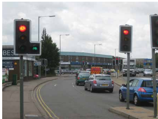
Photo 6.29 – Permanent Green Signal at Bus Gate - Cambridge
