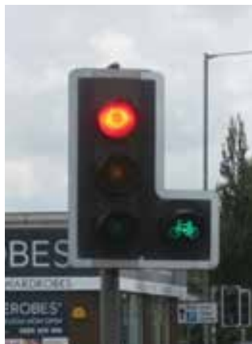
Photo 6.29 – Permanent Green Signal at Bus Gate - Cambridge
