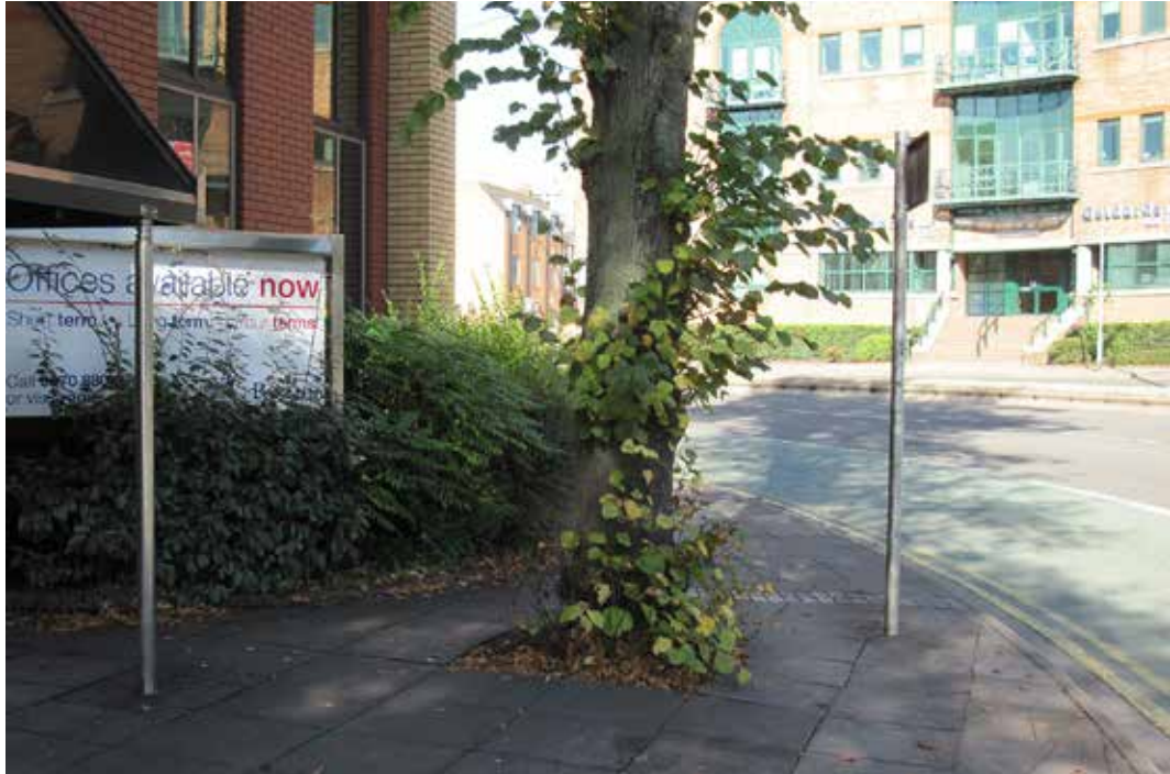
Photo 8.3 – Poorly maintained tree obstructing footway
